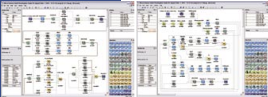
Fig. 4: Visual Applets surface with data flow of HSI segmentation and Sobel edge detection application
